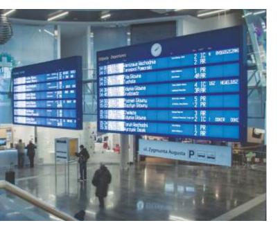
The main parts of the system are information displays, public address devices and clocks. LCD-TFT or (optionally) LED displays can be used. Other system components are infomats and connection search engines, which guarantee optimized access to information. System installation is tailored to site-specific requirements and capabilities, resulting in good reception of broadcast messages. The system is flexible, which allows you to add additional devices if necessary in the future.
